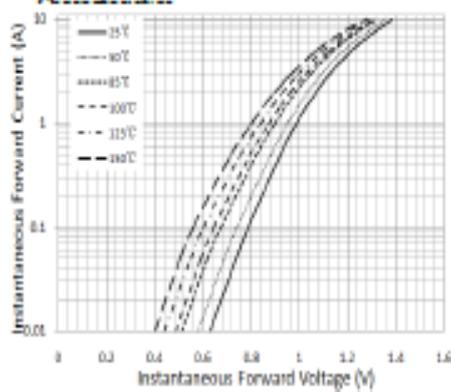
Figure 5. Typical Instantaneous Forward Characteristics
