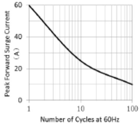
Figure 2. Maximum Non-Repetitive Peak Forward Surge Current
